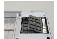
FIGURE 6.13 Adding RAM to a computer is quick and relatively inexpensive. On a laptop, you often gain access through a panel on the bottom. (Shutterstock.com)
